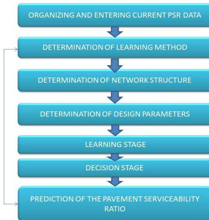
**Figure 4.** Flow chart of the prediction model
